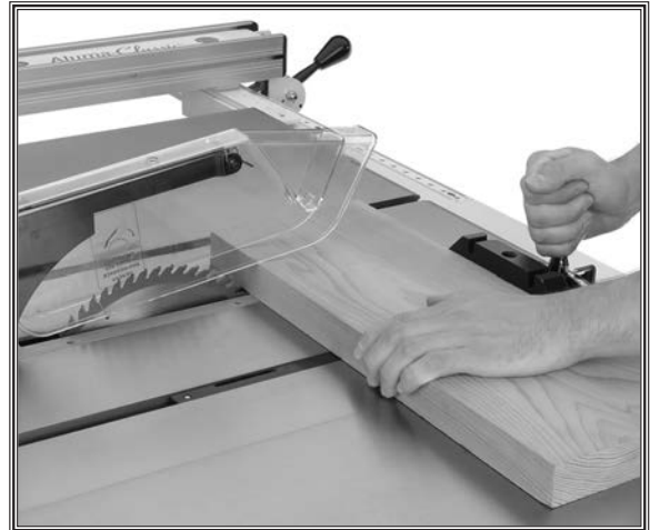
Figure 59. Typical crosscutting operation.
