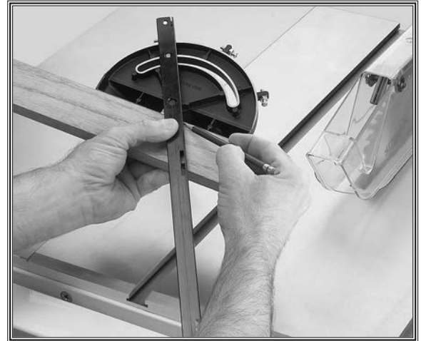
Figure 60. Example of marking miter line.
