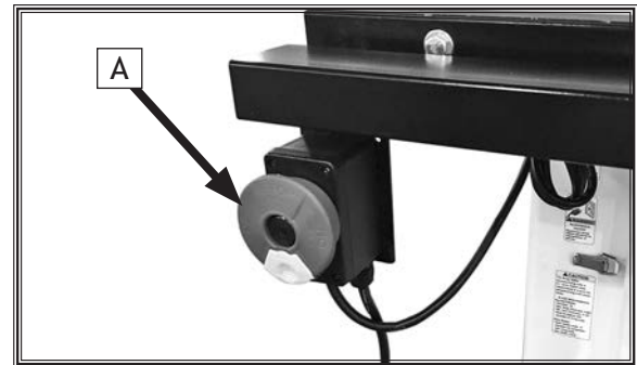
Figure 1. Location of ON/STOP Switch.
