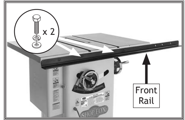
Figure 21. Front rail attached to table.
