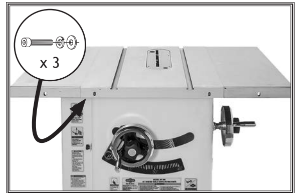
Figure 18. Extension wings installed.
