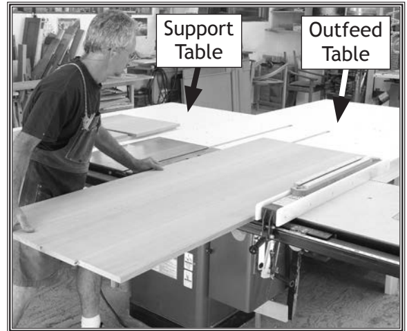
Figure 96. Example of support and outfeed tables.
