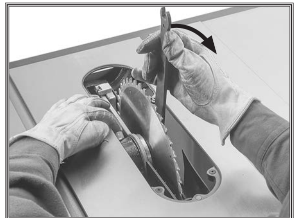
Figure 45. Example of removing table saw blade.
