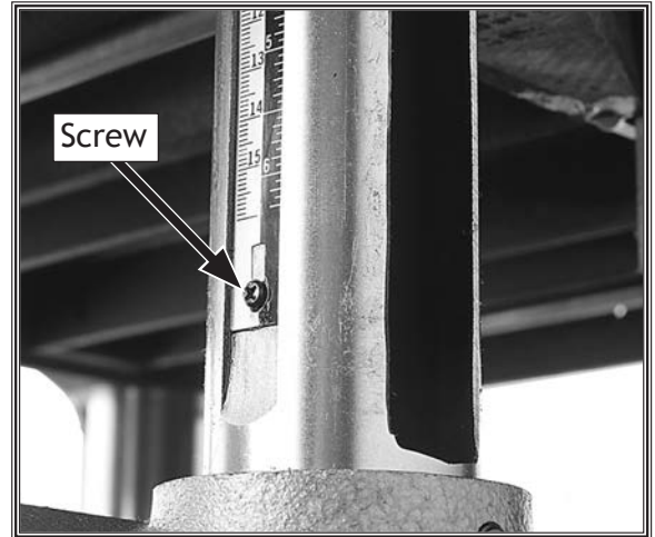
Figure 49. Location of adjustment screw for table elevation scale.
