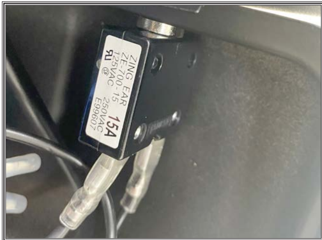
Figure 66. Circuit breaker (W1868 shown).
