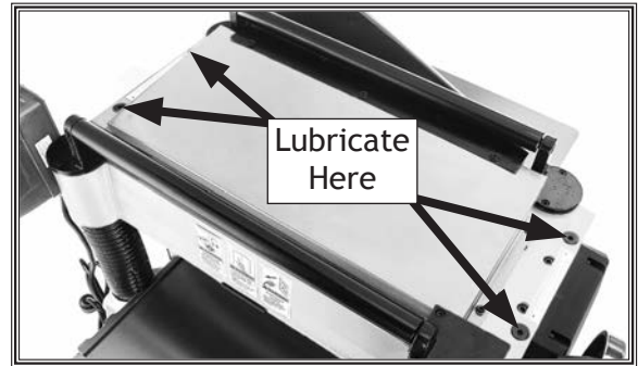
Figure 37. Lubrication locations for feed roller bushings.
