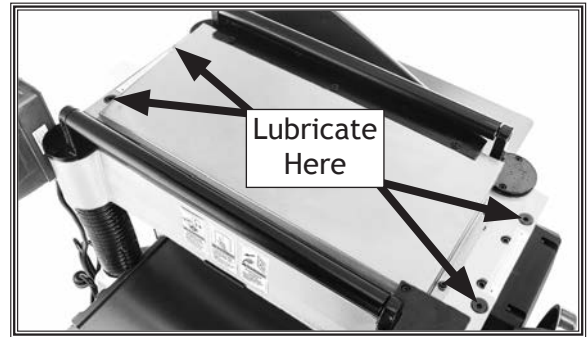
Figure 35. Lubrication locations for feed roller bushings.
