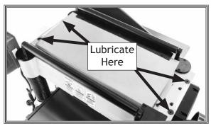
**Figure 35.** Lubrication locations for feed roller bushings.
