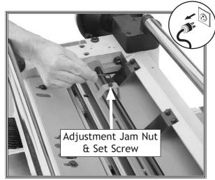
**Figure 49.** Example of adjusting chip breaker height.
