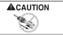
No adapter should be used with the required plug. If the plug does not fit the available receptacle or the machine must be reconnected to a different type of circuit, the reconnection must be made by an electrician or qualified service personnel and it must comply with all local codes and ordinances.
