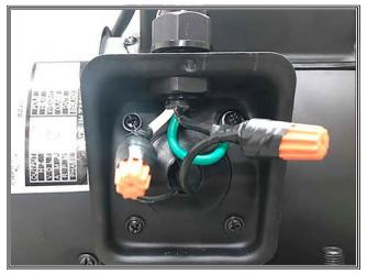
Figure 62. W1862 motor junction box.
