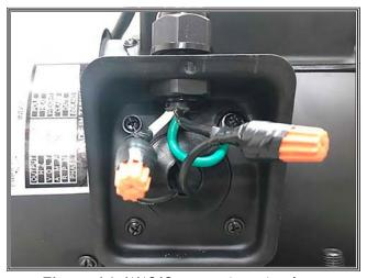
Figure 64. W1863 motor junction box.
