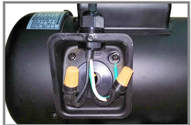
Figure 67. Motor junction box connections.
