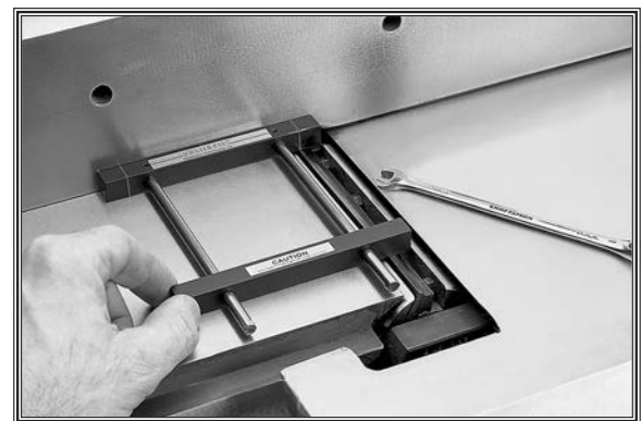
Figure 29. Setting knife height with a Jointer Pal®.
