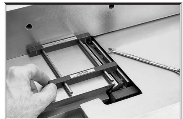
Figure 29. Setting knife height with a Jinter Pal®.
