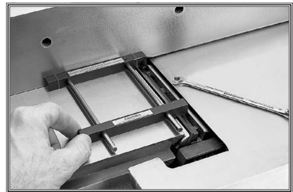
Figure 40. Setting knife height with a Jointer Pal®.
