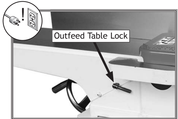
Figure 53. Location of outfeed table lock.
