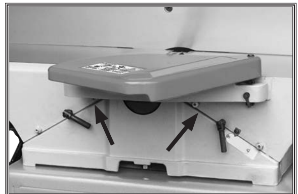
Figure 38. Location to lubricate table ways.
