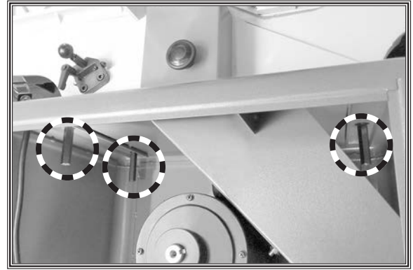
Figure 12. Table assembly secured to stand.
