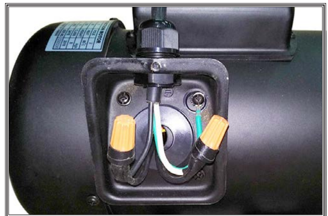
Figure 70. Motor junction box connections.
