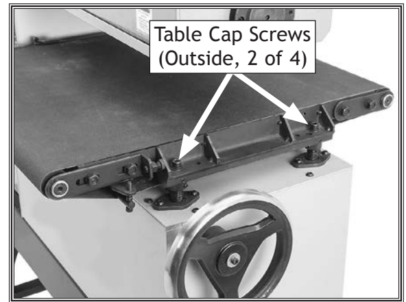
Figure 38. Conveyor belt table outside cap screws.
