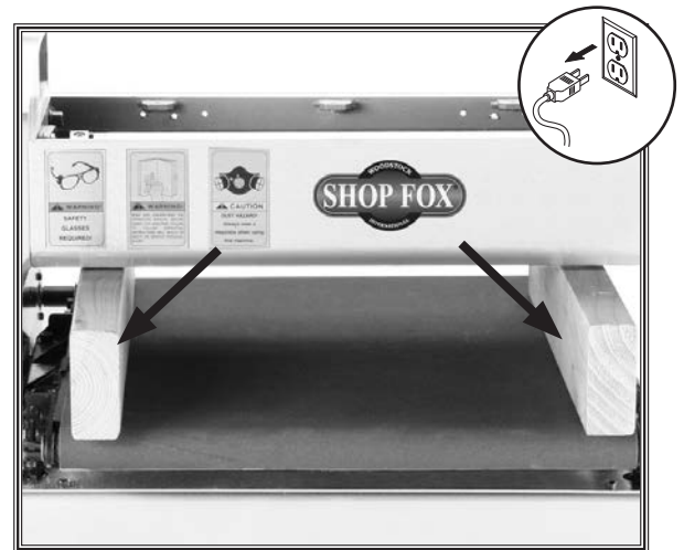
Figure 42. Example of gauge blocks placed under drums.
