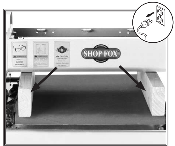
Figure 44. Example of gauge blocks placed under drum.
