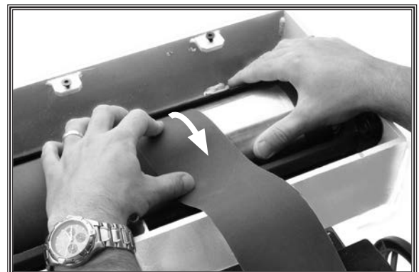
Figure 20. Wrapping sandpaper around drum.
