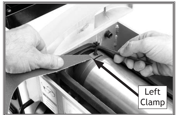
Figure 19. Securing sandpaper in left clamp.
