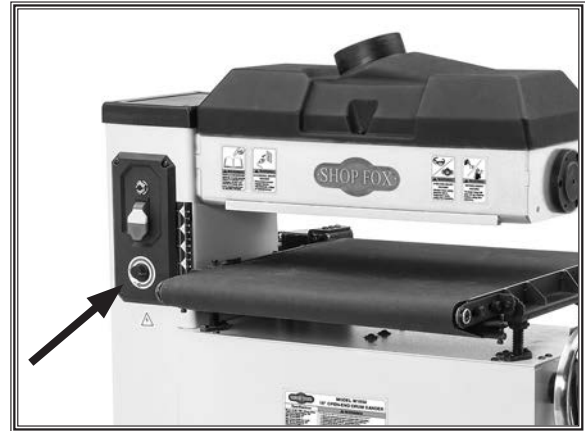
Figure 16. Location of conveyor feed rate dial.
