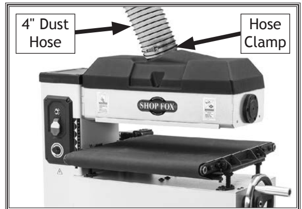
Figure 13. Dust port connected to dust-collection system.
