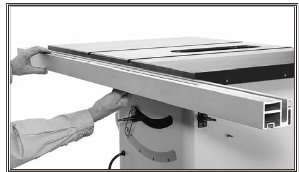
Figure 23. Mounting front fence rail.
