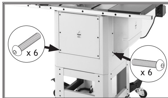
Figure 33. Rear access panel and motor cover installed.
