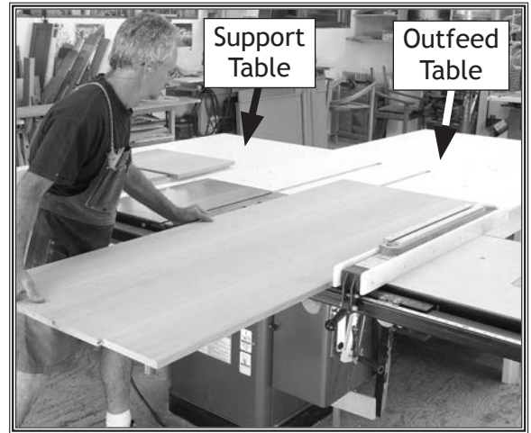
Figure 94. Example of support and outfeed tables.
