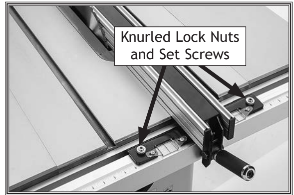
Figure 112. Location of lock nuts and set screws for adjusting fence squareness and height.
