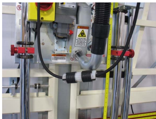
Figure 24: Twist Lock connected
