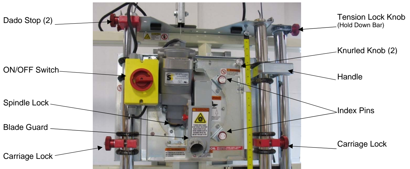
Figure 38: Basic SAW Operating Controls and Components (SR5U & SR5UA)
