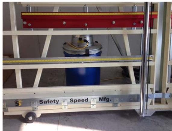
Fig. 78: Midway fence installed
