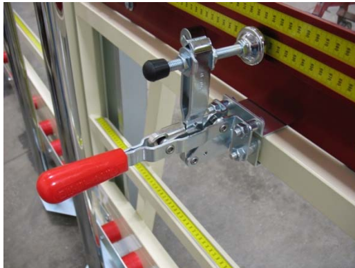
Figure 34: “Upper” Hold-Down Clamp installed
