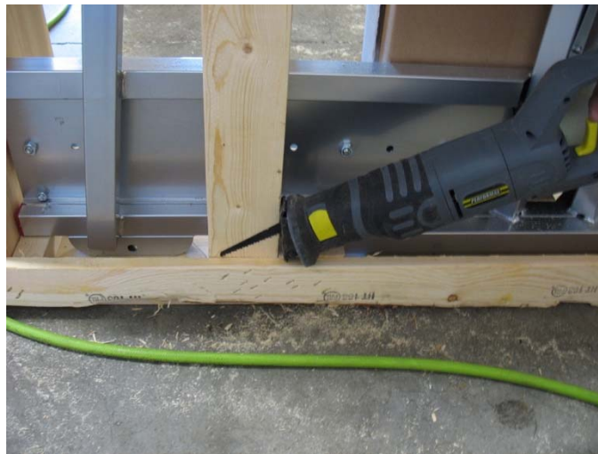
Figure 13: Cutting along base of wood crate, do not cut through (across) base
