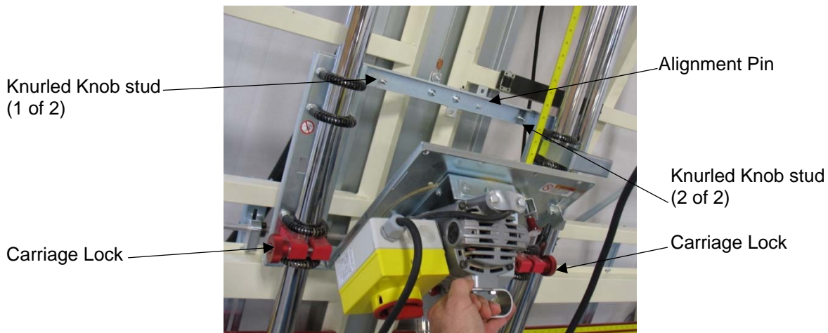
Figure 22: Mounting Saw Plate to Carriage, SR5U shown
