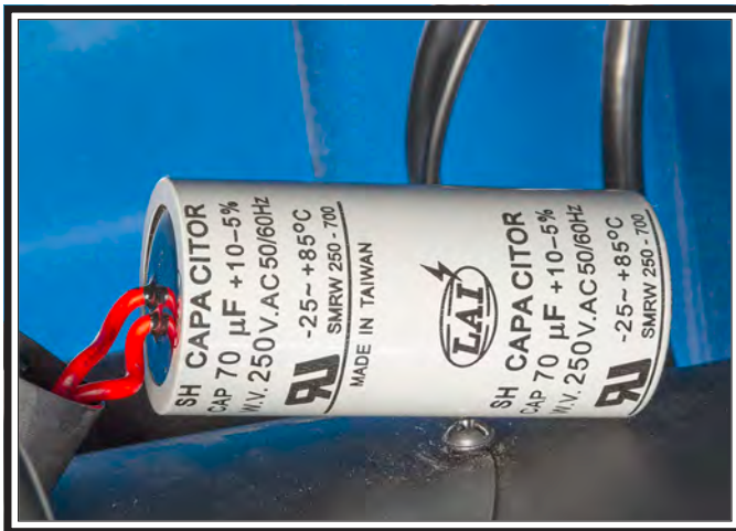
Figure 69. SB1108 run capacitor.
