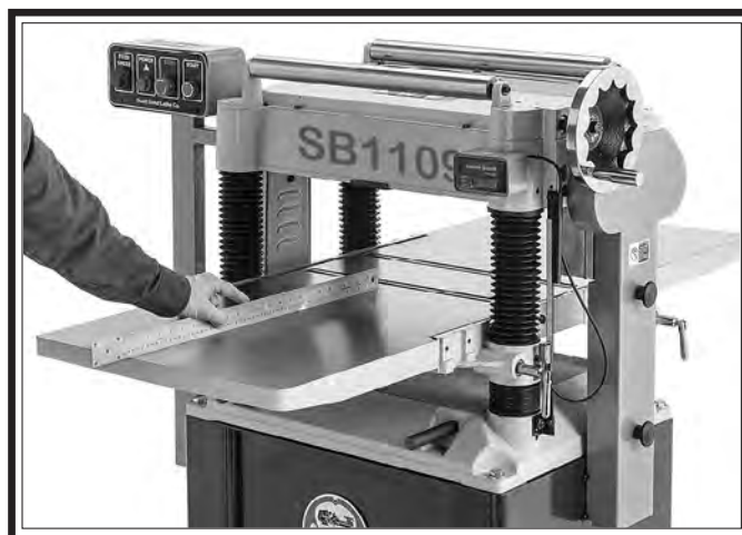
Figure 19. Leveling extension table.
