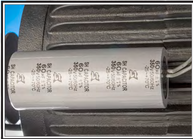
Figure 76. SB1109 run capacitor.
