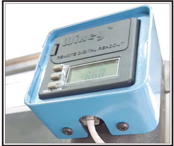
Figure 80. SB1109 height digital readout.
