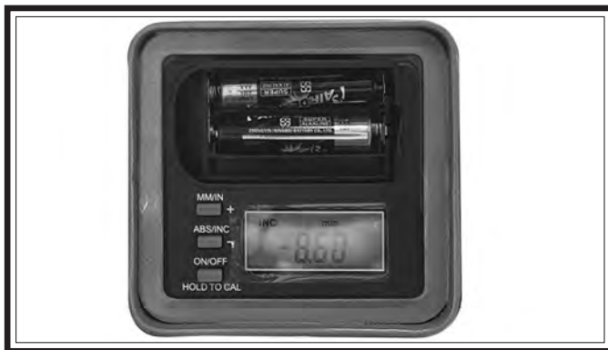
Figure 21. Digital readout batteries installed.
