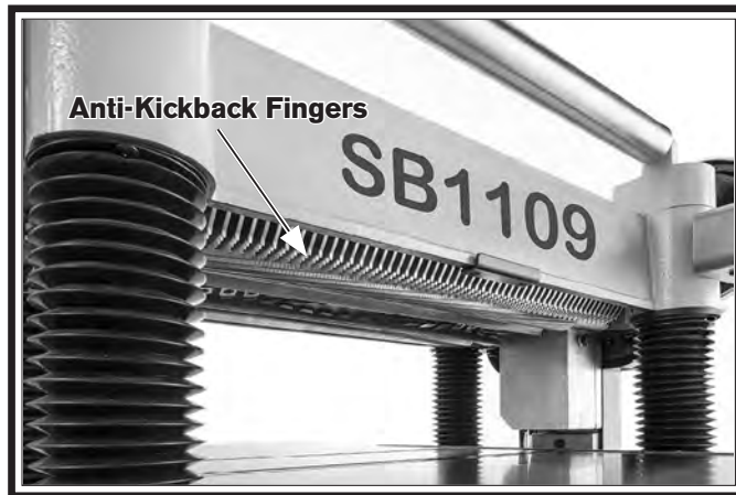
Figure 46. Example of anti-kickback fingers.
