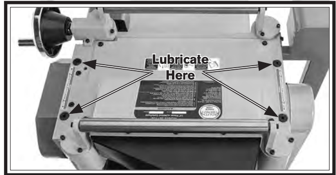
Figure 39. Lubrication locations for feed roller bushings.
