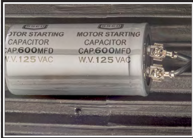
Figure 75. SB1109 start capacitor.
