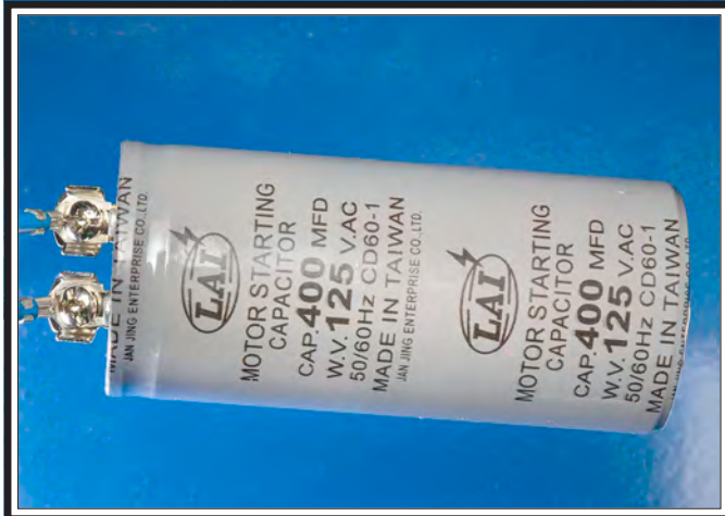
Figure 68. SB1108 start capacitor.
