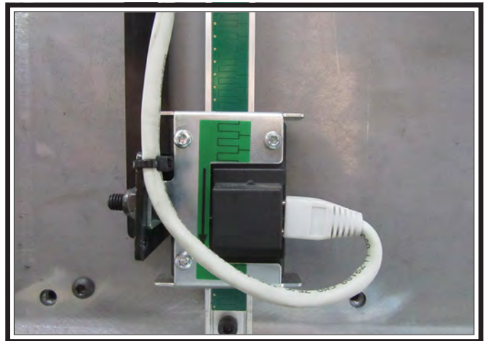
Figure 81. SB1109 DRO height sensor.
