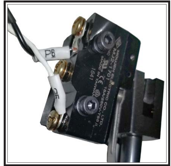
Figure 64. Spindle brake switch (LS7).
