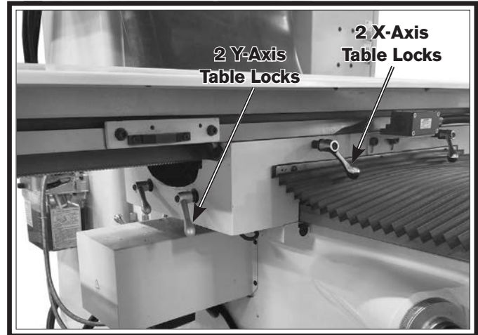
Figure 17. X- and Y-axes table lock locations.
