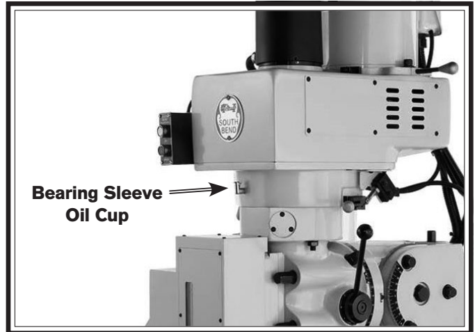
Figure 34. Bearing sleeve oil cup.
