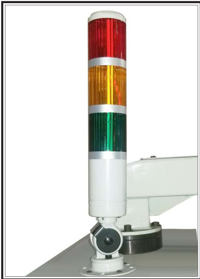
Figure 75. Machine mode indicator light.
