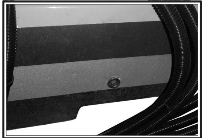
Figure 44. Reservoir drain plug location (rear side of machine base).
