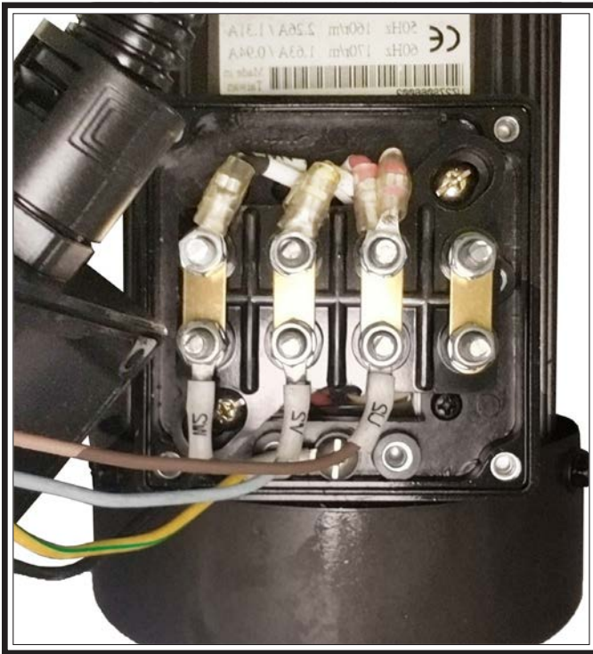
Figure 67. Z-axis motor wiring (220V) (M2).
