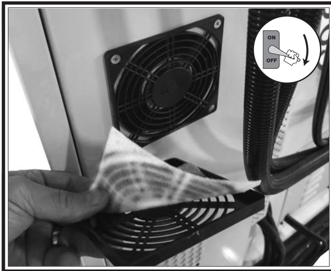
Figure 40. Air filter element.
