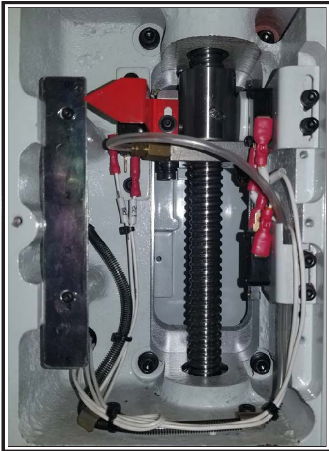
Figure 71. Spindle limit switches (LS3 & LS5).
