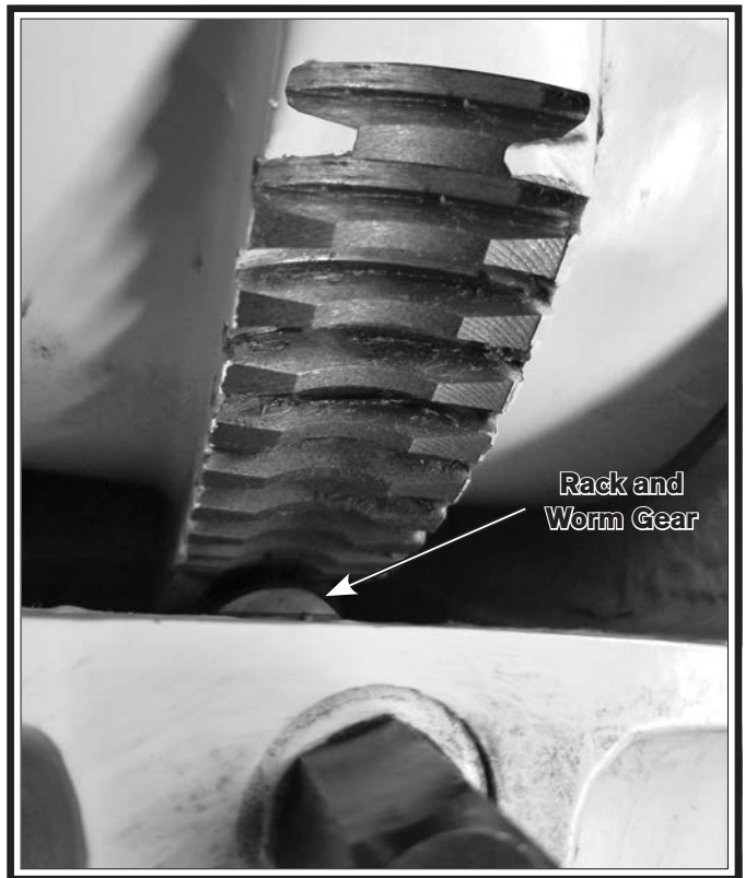
Figure 39. Headstock tilt rack and worm assembly.
