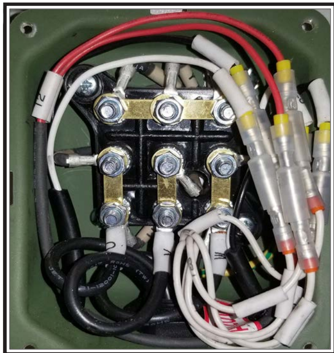
Figure 65. Spindle motor wiring (220V) (M3).
