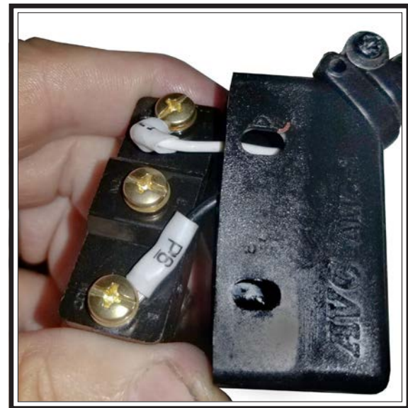
Figure 66. Spindle speed range switch (LS6).
