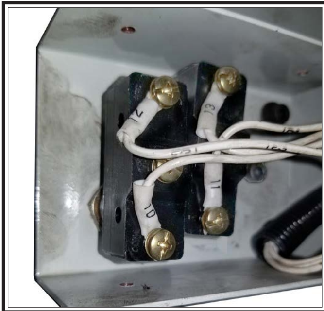
Figure 69. Z-axis limit switches (LS9 & LS10).
