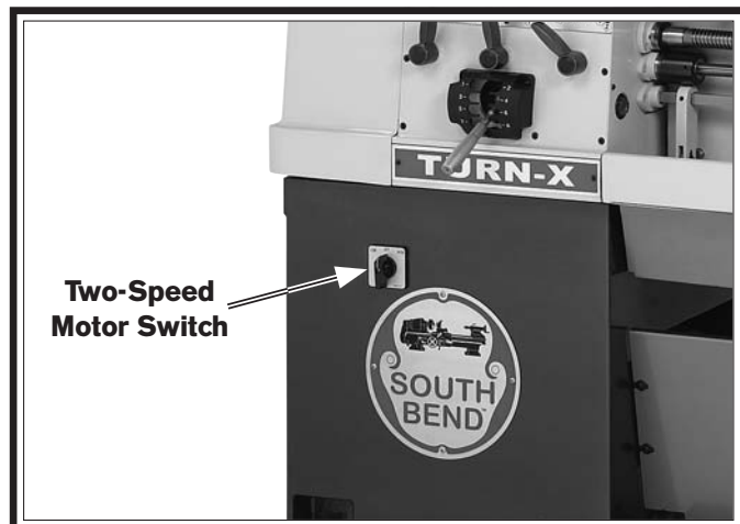
Figure 3. Location of the two-speed motor switch.
