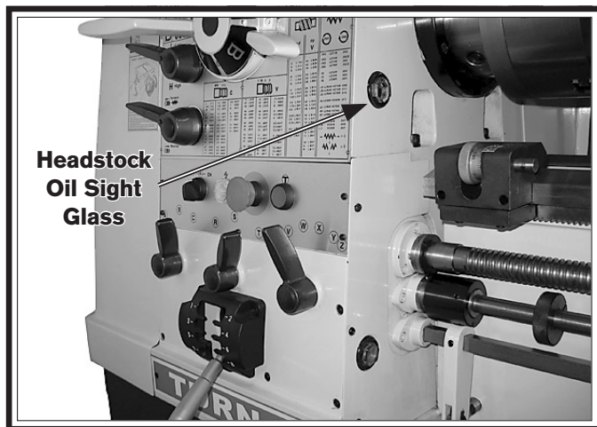
Figure 100. Location of headstock oil sight glass.
