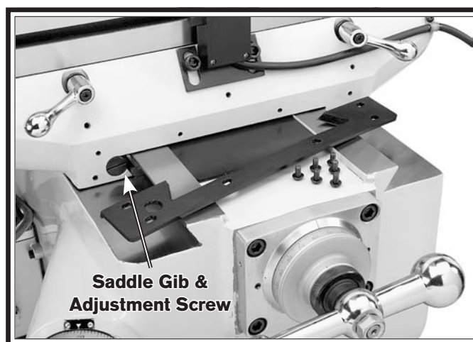
Figure 62. Saddle gib and adjustment screw.
