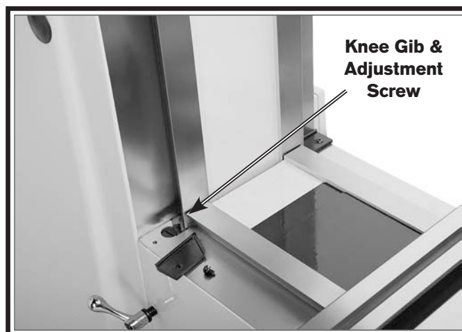
Figure 63. Knee gib and adjustment screw.
