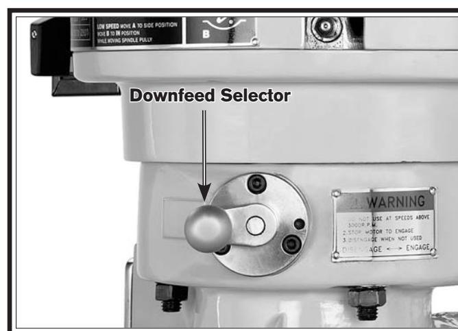
Figure 38. Downfeed selector in the manual (disengaged) position.
