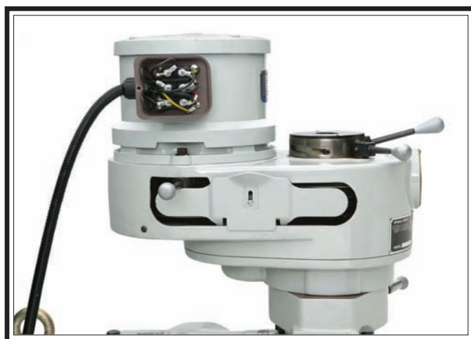
Figure 74. SB1025 Motor junction box.
