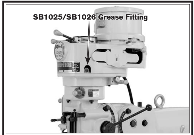
Figure 53. SB1025/SB1026 headstock gearing grease fitting.
