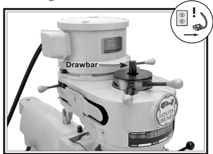
Figure 47. Drawbar loading into the spindle (Model SB1025 shown).
