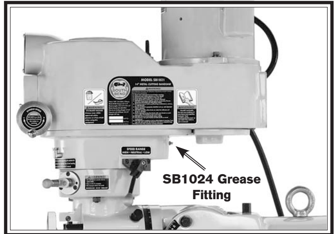
Figure 52. SB1024 headstock gearing grease fitting.
