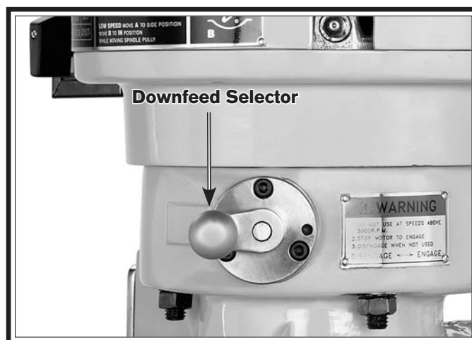
Figure 38. Downfeed selector in the manual (disengaged) position.
