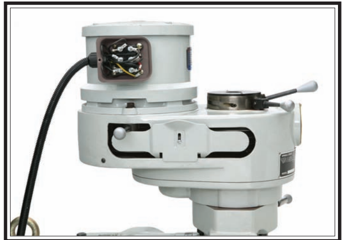
Figure 74. SB1025 Motor junction box.
