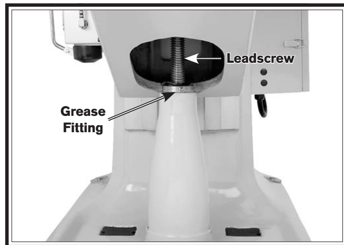
Figure 56. Table elevation leadscrew and grease fitting.
