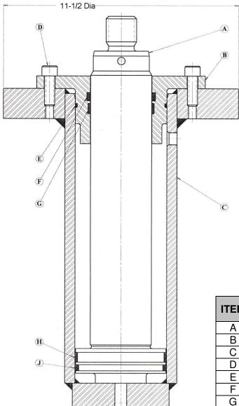
25 ton Workhead 4-1/2" Dia. Bore 3" Dia. Rod 10-1/4" Actual Stroke 10" Rated Stroke Total Wt. = 127#
