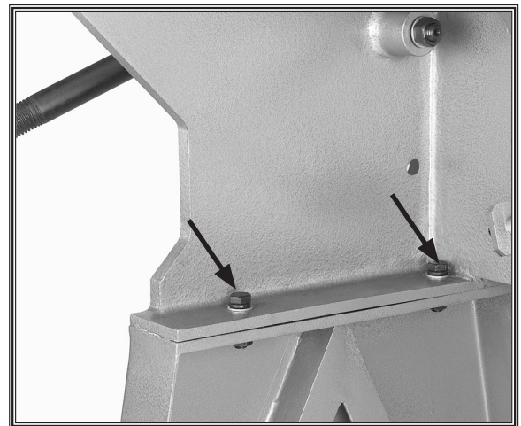
Figure 9. Main body mounted to supports.
