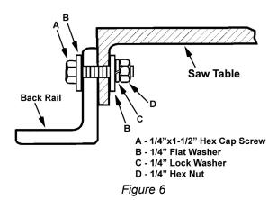
**Important:** If you are installing an optional wood extension table on your saw, it should be installed first **before** mounting the guide tube. This will prevent having to mount and align the guide tube twice.
