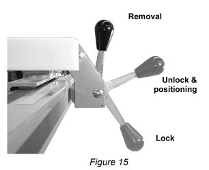
Leveling Fence to the Saw Table
