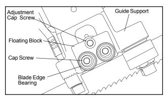
Figure 21: Blade edge bearing replacement
