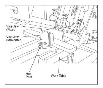
Figure 9: Securing the Workpiece
