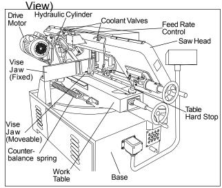
Figure 2: Key Features (Rear View)
