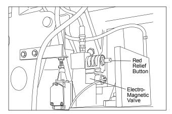
Figure 6: Lowering head with power off
