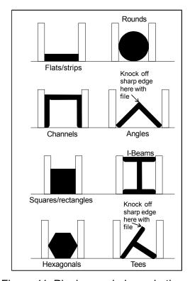
Figure 11: Placing workpieces in the vise
