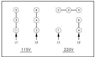
Figure 24: Connection diagram for 1ph motor
