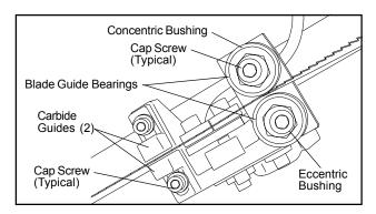
Figure 20: Carbide blade guides and guide bearings
