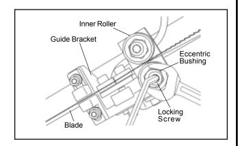
Figure 14: Adjustment of guide bearings
