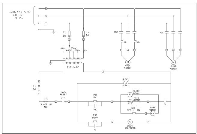
Figure 25: Model 7040M cut-off saw wiring diagram
