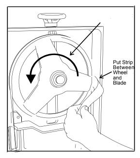
Figure 13: Checking blade-to-wheel clearance using paper strips
