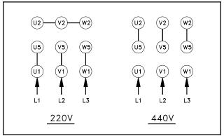
Figure 26: Connection diagram for 3ph motor
