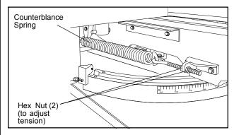
Figure 18: Counterblance Spring Adjustment
