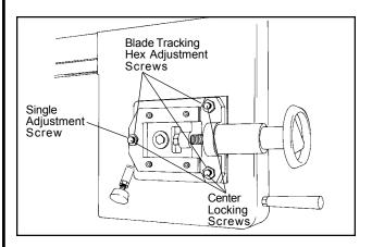
Figure 12: Blade tracking and tensioning Factory or Field Procedure
