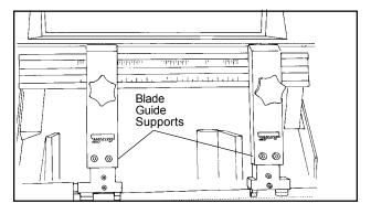
Figure 19: Blade guide supports
