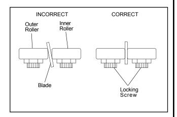
Figure 15: Blade -to-bearing orientation
