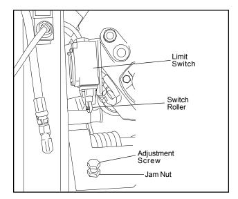
Figure 15: Limit switch adjustment
