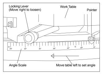
Figure 7: Quick-Acting Swivel-Head Lock
