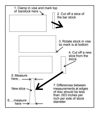
Figure 16: Cutting a test disc
