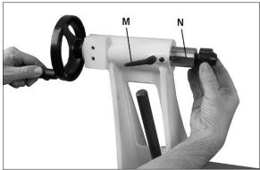
Figure 7-9: installing live center
