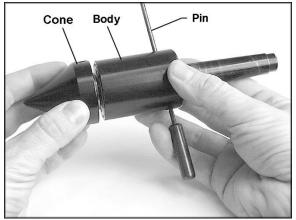
Figure 7-10: removing cone from live center
