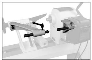
Figure 5-7: installing comparator (optional)
