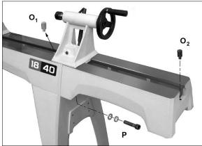
Figure 5-6: installing bed extension (optional)
