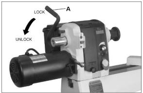
Figure 7-1: headstock movement
