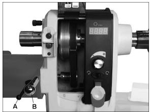
Figure 7-13: speed range adjustment
