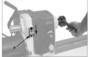
Figure 7-11: spindle lock and face plate
