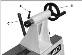
Figure 7-3: tailstock movement
