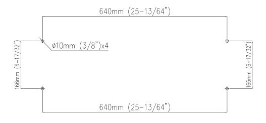
Figure 2 Clearance hole spacing for mounting lathe
