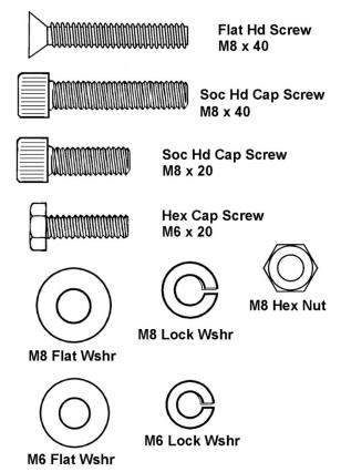
Figure 5-3: contents of hardware package
