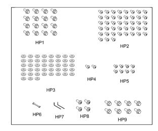
Figure 5-2: # **PM2200-HP-1** hardware package contents (not to scale)
