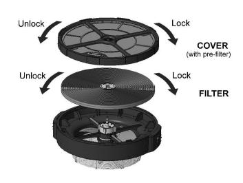
Figure 8-4: Filter replacement
