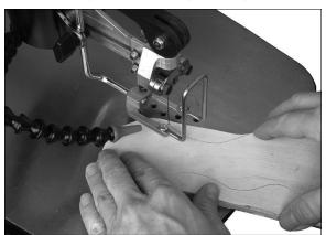
Figure 10-2: contour cutting
