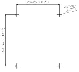
Figure 5-1: JWSS-18B mounting hole pattern
