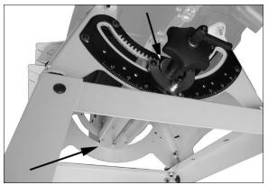
Figure 11-1: lubrication (shown with optional stand)
