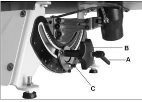
Figure 9-1: arm tilt adjustment
