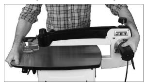
Figure 7-4: correct lifting
