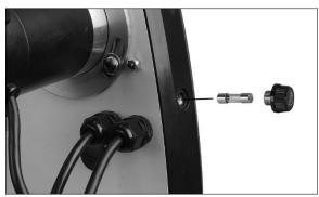
Figure 11-2: fuse inspection
