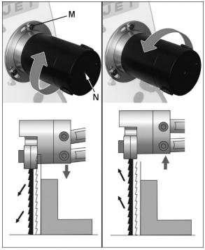
Figure 9-11: blade oscillation
