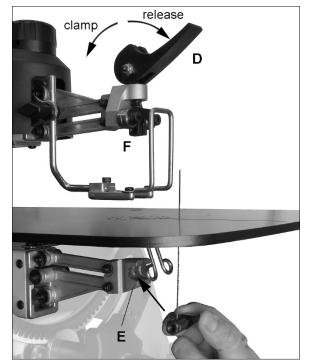
Figure 9-3: installing blade into guides
