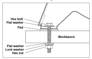
Figure 7-6: bench mounting (fasteners not included)
