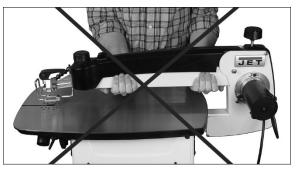
Figure 7-3: INCORRECT lifting
