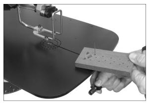
Figure 9-4: installing blade with workpiece
