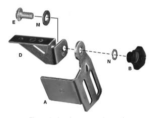
Figure 3: brackets to spark guards
