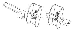
Figure 9 – switch lockout (padlock not provided)
