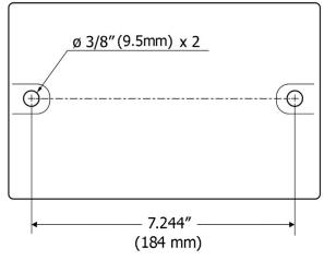
Figure 2: mounting holes
