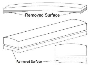
6. To initiate a cut, stand near the infeed table, slightly behind the cutterhead. Use left hand to push firmly on stock against the fence and infeed table, and use right hand to feed the stock from the back. Use push blocks whenever permissible.
