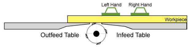
8. As left hand approaches the cutterhead, lift it up and move across the cutterhead to avoid accidental contact. Put left hand on stock that sits on the outfeed table, and continue to feed. Maintain control of stock with right hand while repositioning left hand.
