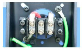
4. Insert power cord through strain relief. The strain relief can be temporarily removed from junction box to make this task easier.
