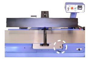
2. The guard must be installed as low as possible without scratching the table.
