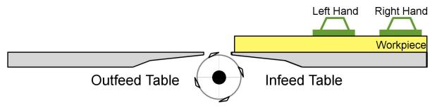
7. Feed a small section of stock across the cutterhead with pressure against the fence and the infeed table.
