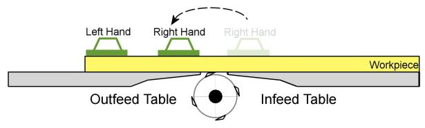
10. From this point on, continue feeding only on outfeed table until the entire length of stock has moved across the cutterhead. Maintain feed rate to produce smooth cut with no burnt marks.
