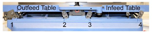
7. Locate and loosen the set screws for locking the eccentric nuts as shows in the pictures:
