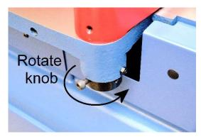
**NOTICE**: There are four screw holes on the knob. If the cap screw gets in the way while the knob rotates, relocate the screw and tighten when the knob is rotated to the proper position.
