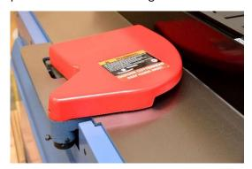
3. There is spring-loaded knob at the bottom of rabbeting table. It has a cap screw which grabs the cutterhead guard shaft and keeps the guard pushing against the fence.
