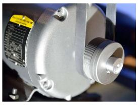
If the belt is too tight to remove, temporarily loosen the upper mounting bolts (#2). Raise the motor to loosen the belt, and remove it from the pulleys.
