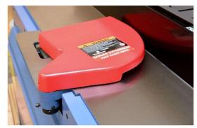
WARNING: If cutterhead guard needs adjustment, <u>STOP HERE</u>. Have the guard adjusted before resuming the test run.
