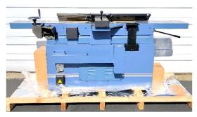
2. Remove all six cap screws from control panel post.
