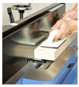
Feed the workpiece through completely across cutterhead while keeping it firmly against fence and tables during the entire cut.
