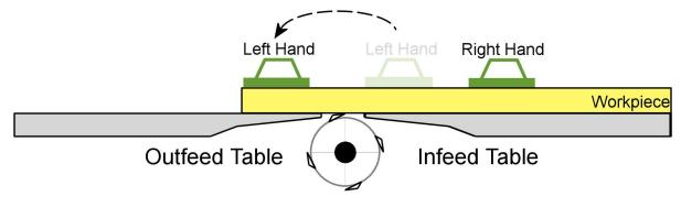
9. As the right hand approaches the cutterhead, reposition right hand as shown in the diagram. Operator should move forward and continue feeding next to the outfeed table. Maintain control of stock with left hand while repositioning right hand.
