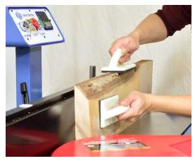
7. Follow steps [6-10] in "Surface Planing" for feeding stock through the jointer. Repeat the process until the entire edge is jointed flat and square.
