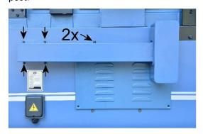
3. Raise the control panel to its operational position, then remount it back to the cabinet.
