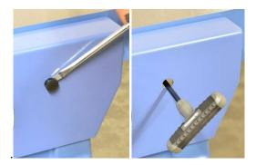
6. This picture shows the jointer with the parallelogram mechanism exposed. Table parallelism /coplanarity can be adjusted by rotating the eccentric nuts on the shafts [1-4]. There is a pair of eccentric nuts located on each end of these shafts.
