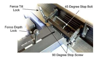
The fence can be retracted and raised above the table to provide additional clearance for servicing the cutterhead.
