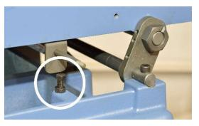
4. The stop nut for finishing passes is located below the infeed table, near the height adjustment worm gears. This stop nut should stop the table with 1/32" depth of cut. Loosen the jam nuts when making adjustments.
