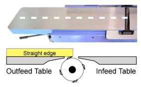
6. When outfeed table height is properly set, cutters should be barely scraping the straight edge when cutterhead rotates. Follow the next section to make adjustments as needed.
