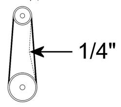
4. If V-belt tension needs to be adjusted, loosen both lower motor mounting bolts (#1). Lower the motor until proper belt tension is reached. Secure the motor mounting plate by tightening both upper mounting bolts (#2), and the lower mounting bolts.
