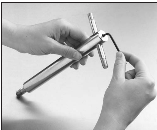
Figure 11. Tightening setscrew with hex key.
