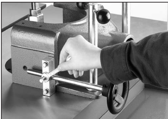
Figure 15. Tightening bolt into shaft groove.
