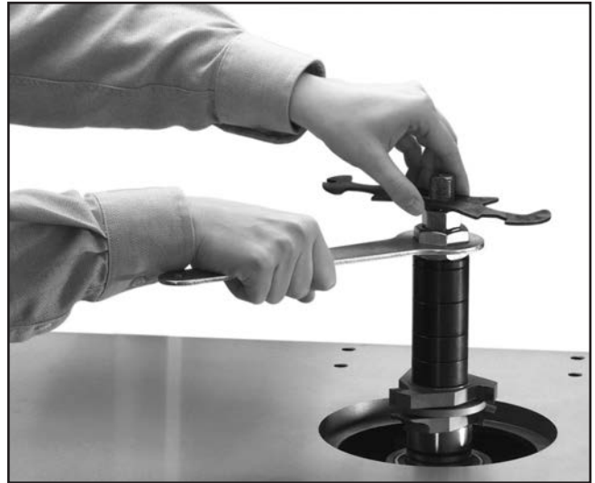
Figure 30. Tightening spindle nuts.
