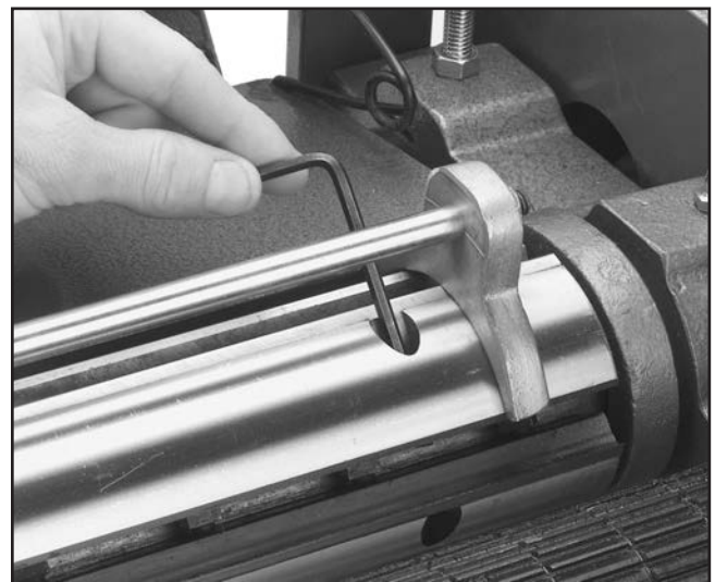
Figure 8. Adjusting knife height.
