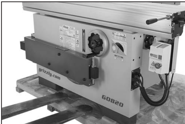
Figure 16. How to insert forks for lifting table saw off pallet.
