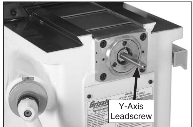
Figure 79. Ball handle, ring, and key removed from Y-axis leadscrew.
