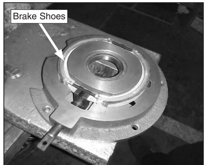
Figure 102. Lower pulley, shaft, and bearing sleeve removed to expose brake shoes for inspection/replacement.
