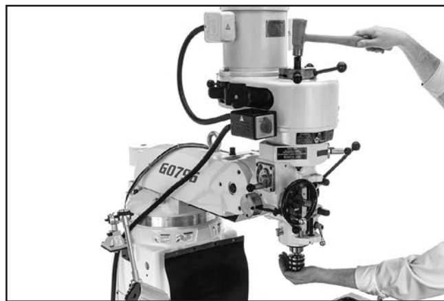
Figure 49. Tapping drawbar to unseat tool taper (G0796 shown).
