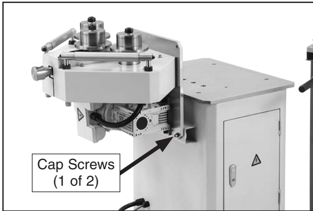
Figure 7. Location of cap screws that secure headstock in horizontal position.
