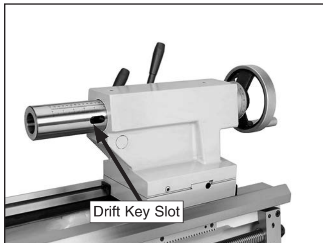
Figure 39. Drift key slot in the side of the quill.
