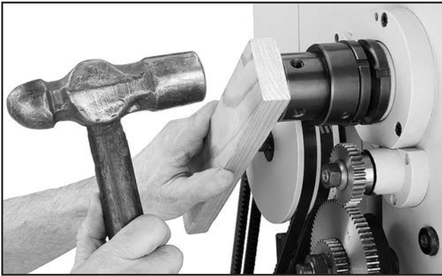
Figure 143. Unseating spindle bearings to introduce spindle end-play.
