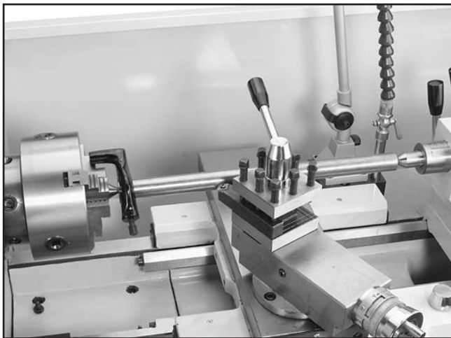
Figure 50. Example photo of a workpiece mounted between the centers.
