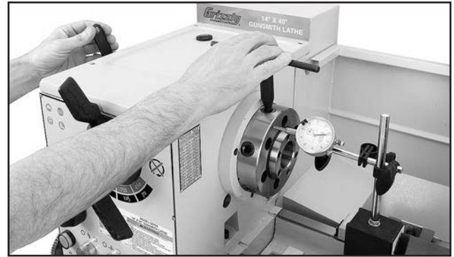
Figure 145. Adjusting spindle bearings.
