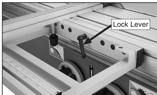
Figure 106. Location of crosscut table lock lever.
