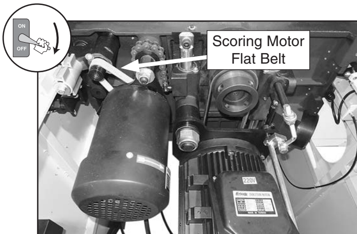
Figure 150. Location of scoring motor flat belt.
