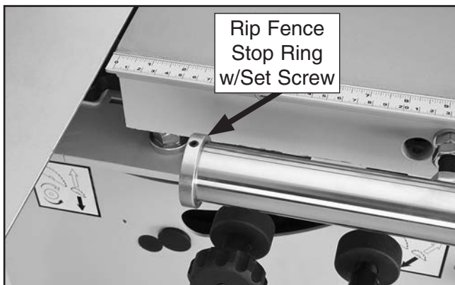
Figure 41. Rip fence stop ring attached to rail.
