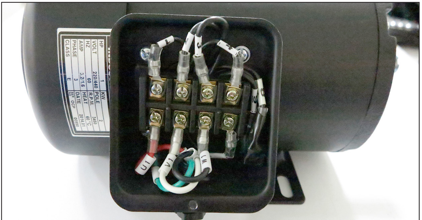
Figure 175. Scoring motor wiring.
