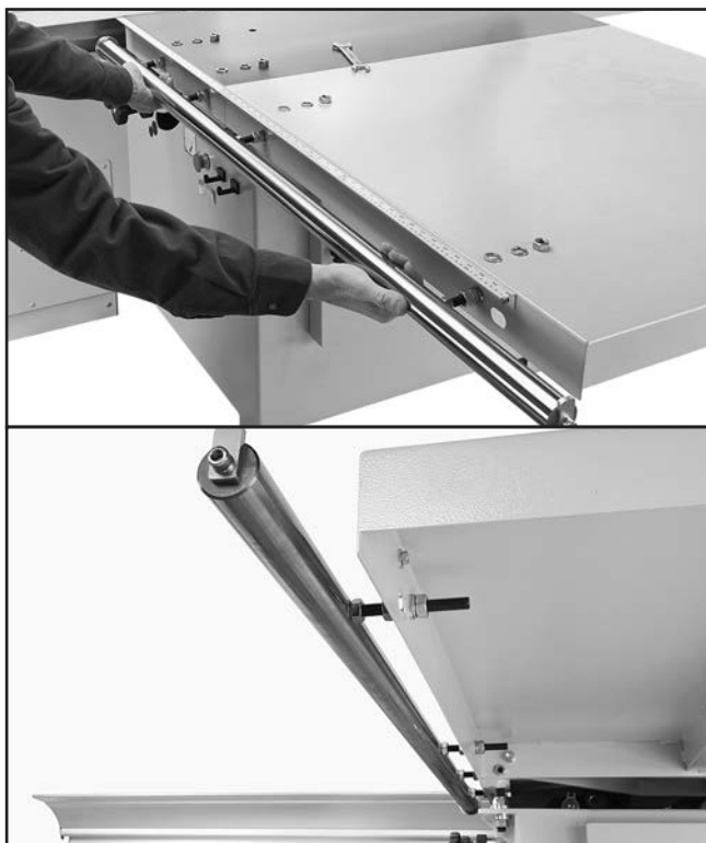
Figure 33. Installing the rip fence rail.
