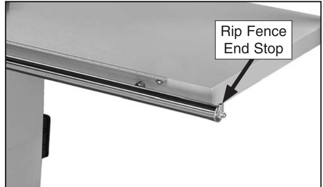
Figure 42. Rip fence end stop attached to rail.
