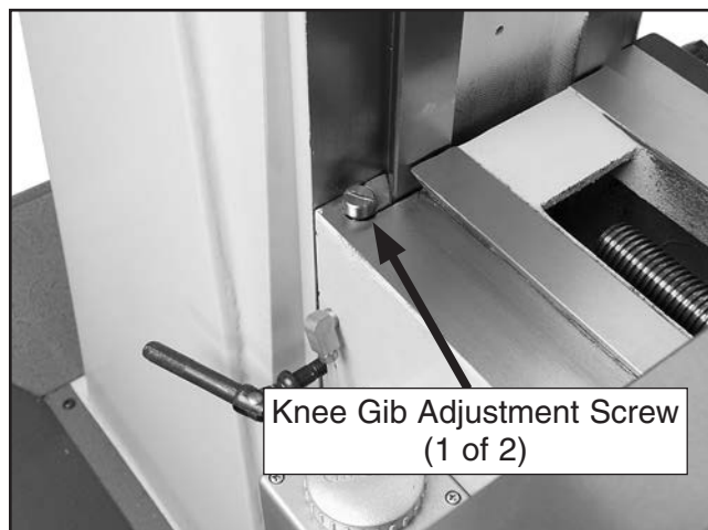
Figure 45. Knee gib adjustment screw (1 of 2).
