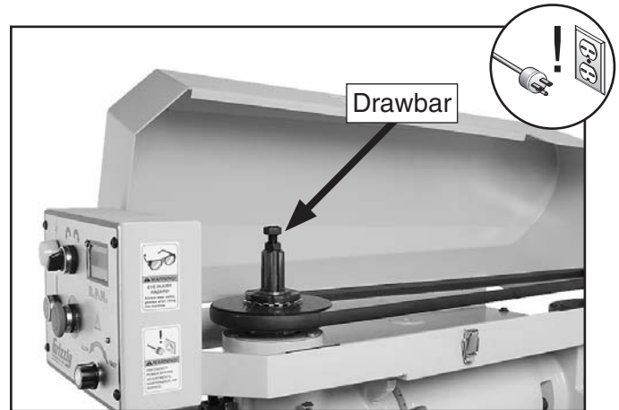
Figure 27. Drawbar inserted through the top of the spindle.
