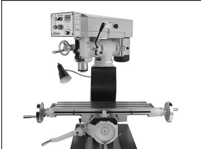
Figure 20. Head and turret rotated 45° to the left.
