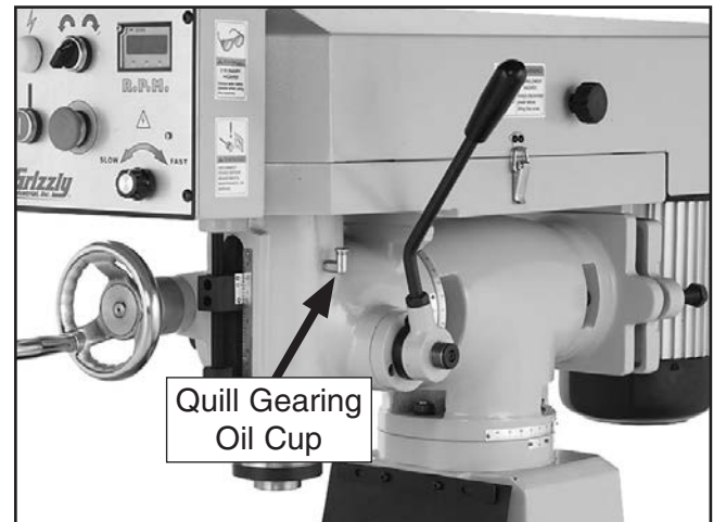
Figure 37. Quill gearing oil cup.
