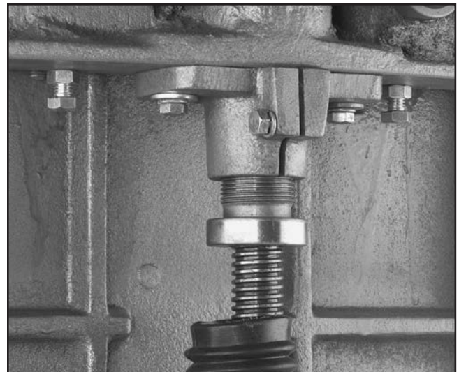
Figure 12. Column adjustment flange underneath table.
