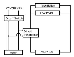
The on/off switch turns power on to both the electric motor and the valve coil circuit. The switch must be 1 HP rated.
