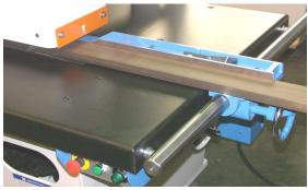
When using the right feed track: The wood goes a little bit rightward. With the supporting plate on its right, it produces excellent parallelism. It is ideal for specific size cutting.
