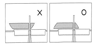
E. If the wood piece is not deformed, have the stretched side face downward to contact with the chains.
