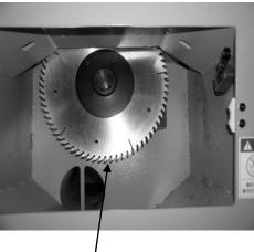
Be sure the saw blade is installed in the correct direction.
