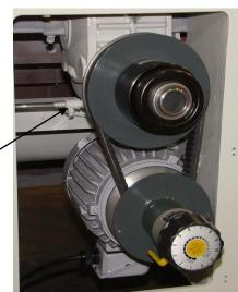
Pour new lubricant from the port on the top. The capacity is about a half of the oil-mirror.
