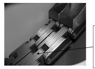
Please check this window daily to make sure whether oil exists at the bottom of the feed track. If no oil exists or oil spreads unequally, please stop the machine immediately and ask for repair.
