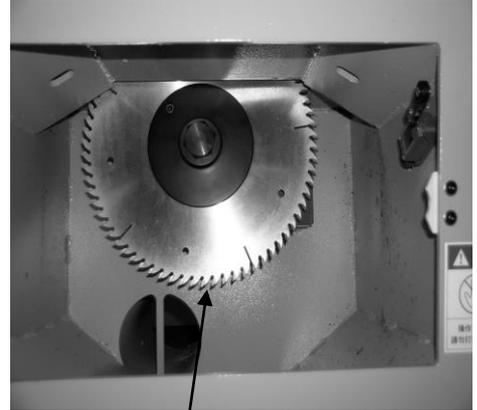
Be sure the saw blade is installed in the correct direction.
