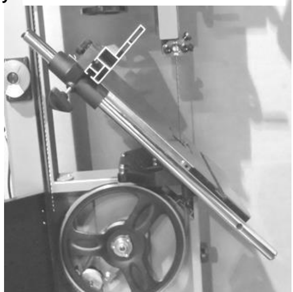
Side guides adjusted with ceramic just behind the gullet
