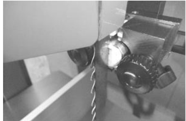
Back guide touching back of the blade
