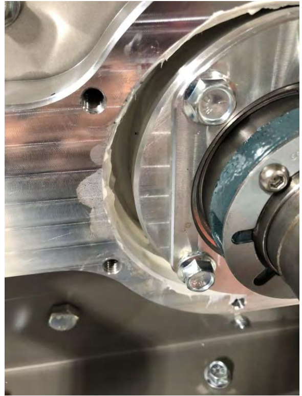
Grease At Rear Of Slide
