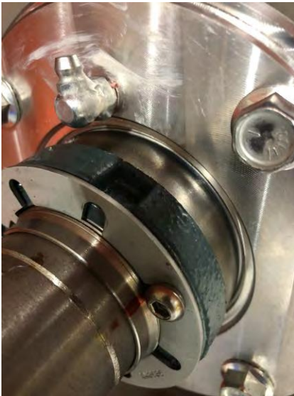
Grease Going Out The Back Seal
