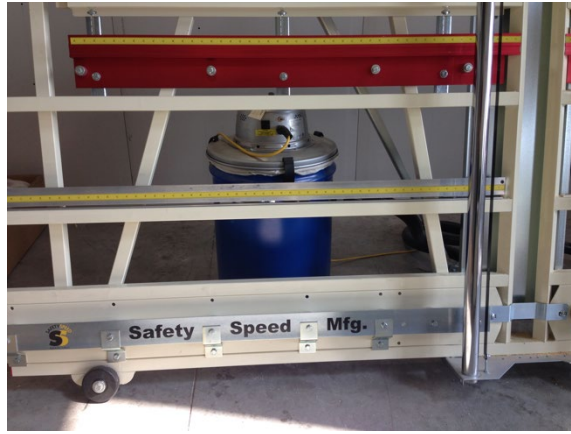
Fig. 59: Midway fence installed
