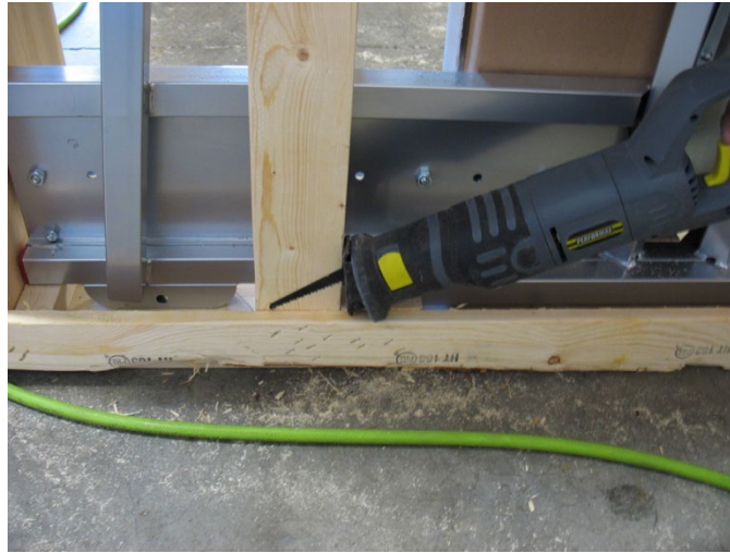
Figure 8: Cutting along base of wood crate, do not cut through (across) base
