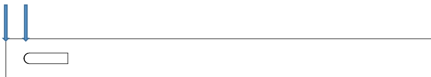
Figure 16: Web dimension, 5/8" minimum
