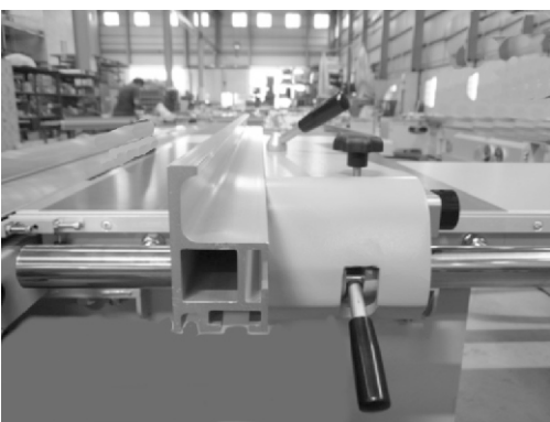
Above drawing is the position of aluminum fence at 90 degree cutting.
