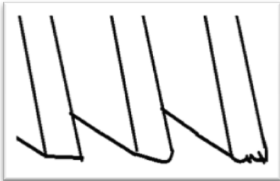
New blade With Without Break-in Break-in
