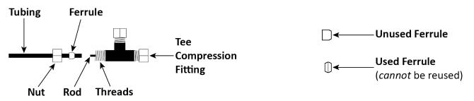
**Important**: *Ferrules can only be tightened once*. When you tighten the Nut on the Threads, the Ferrule is compressed; it literally changes shape and *cannot* be used again.
