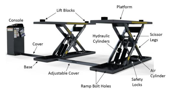
MDS-6EXT shown without Ramps. Power Unit and Flow Divider are inside the Console. Air and Hydraulic Hoses are routed under the two Covers.
