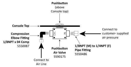
Pushbutton is above the Console top panel, all other components are under the Console top. Drawing not to scale. Not all components shown.
