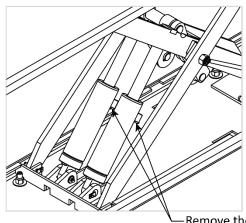
Remove the four plastic shipping plugs from the Cylinder Return Ports
