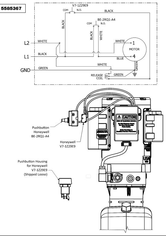
Refer to the wiring schematics below to connect power and the Console control pushbuttons. A Power Disconnect Switch and an External Thermal Overload Protection device in accordance with the National Electrical code and CE code Part 1, *must be provided by a licensed, certified Electrician*. Wiring providing power to this unit must be rated for 3 H.P., 1 Phase, 208-240 Volt, 50/60 Hz., 30 Amps.
