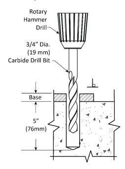
Use a Carbide Concrete Drill (conforming to ANSI B212.15).
