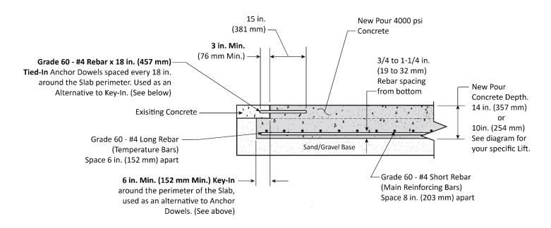
The second method uses Anchor Dowels and the New Pour is said to be **"Tied-In".** Anchor Dowels are made from **#4 Rebar x 18 inches / 457 mm long.** These Anchor Dowels are then embedded **3 inches / 76 mm** minimum into the existing concrete and spaced **18 inches / 457 mm** apart around the perimeter of the New Pour. See figure above.
