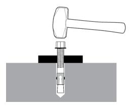
Even using a hammer or mallet, the Anchor Bolt should only go into the hole part of the way; this is normal. If the Anchor Bolt goes all the way in with little or no resistance, the hole is too large.
