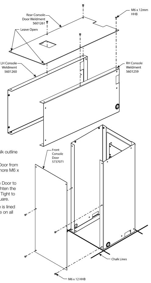
**Note**: There are four mounting holes in the bottom flange of the Console. You only need to anchor two of the four holes. BendPak recommends installing them diagonally from each other; one in the front right, the other in the left rear, for example.
