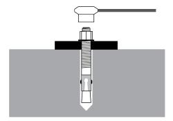
**Important**: Do *not* use an impact wrench to torque the Anchor Bolts.
