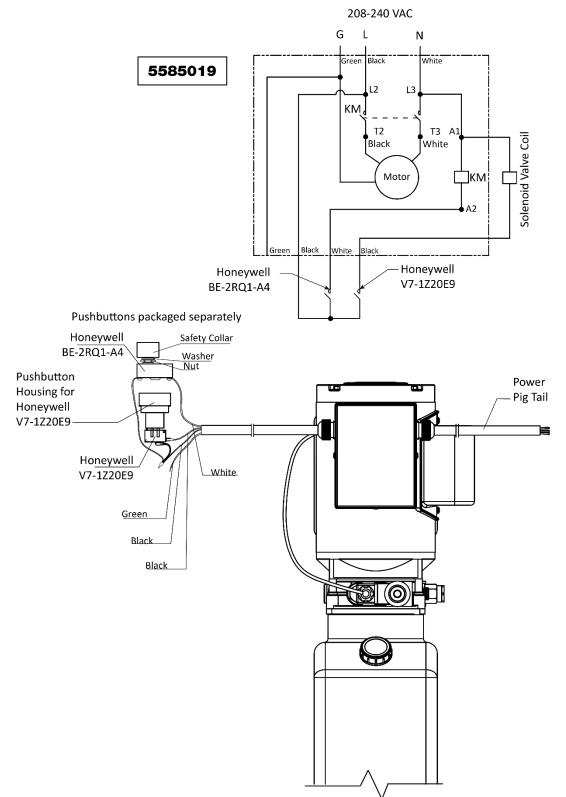
Refer to the wiring schematics below to connect power and the Console control pushbuttons. A Power Disconnect Switch and an External Thermal Overload Protection device in accordance with the National Electrical code and CE code Part 1, *must be provided by a licensed, certified Electrician*. Wiring providing power to this unit must be rated for 1 H.P., 1 Phase, 110/120 Volt, 50/60 Hz.
