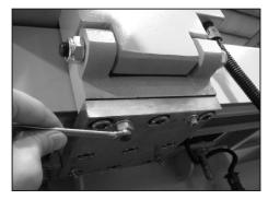
Step 4 : Use the open wrench 8 to adjust the screw to make the fence parallel to main saw blade. (See the left drawing)
