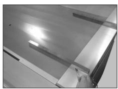
Step 2 : Adjust the gap between electric rip fence and main working table and then tighten the screw shown in Step 1.(Electric rip fence must be in the gap 0~0.1mm under the main working table.)
