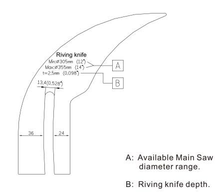
★Prior to setting the riving knife, check whether it matches the saw blade diameter and body thickness.
