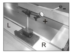
Step 5 : Use the measuring gauge to measure parallelism of the fence and the main saw blade.
