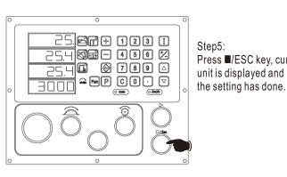
Step5: Press ■/ESC key, current unit is displayed and
