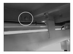
Step 1 : Put on the screw which is used to electric rip fence, working table and extension table (See the left drawing).
