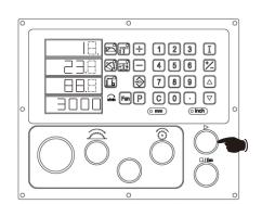
Step 5: Press key, the indicator lights up, display panels stop flashing, and movement starts toward the set position.
