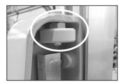
Step 6 : Adjust the eccentric wheel at front end of the fence base to make the fence base parallel to the working table.
