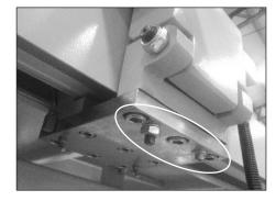
Step 3 : Put on the screw which is used to fasten the fence base and the electric rip fence. (See the left drawing)
