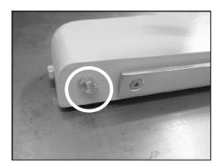
Step 7 : Adjust the eccentric wheel at the side of the fence base to make aluminum fence parallel to the wokring table. At this time, assembly of electric rip fence is completed.
