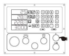
Step 12: Press ▶ key, the start indicator lights up, the display stops flashing, the r indicator goes out, and movement starts toward the set position.
