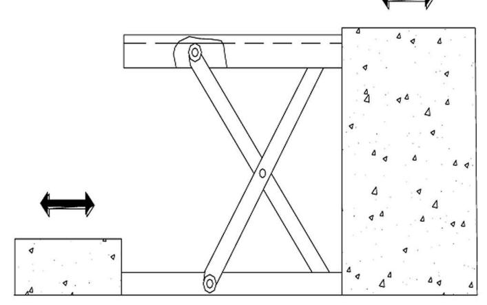
Loading/unloading at the fixed arm end
